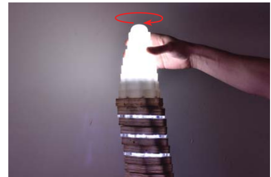
Rotating Stalaglight's lampshade again will fade on all three rows of LEDs in sequence and finally turn the main bulb on to the highest brightness level. Another rotation will turn Stalaglight off.
