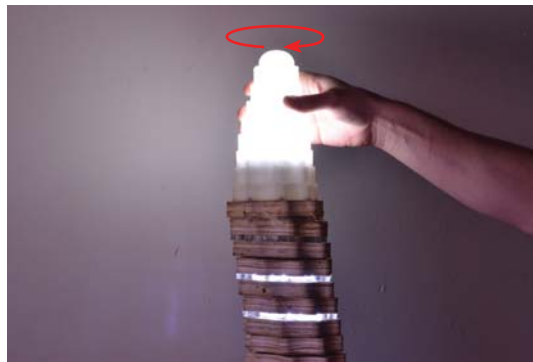
Rotating Stalaglight's lampshade 90° clockwise again should make the first two rows of LEDs fade on in sequence, and the main bulb should turn on to the second brightness level.
